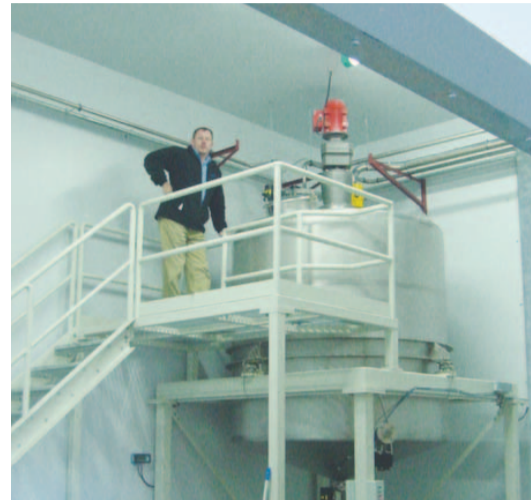
■ Pacific Urethanes managing director Paul Blakeley looks over the company's new six-tonne blending system, which is certified to blend cyclopentane.
